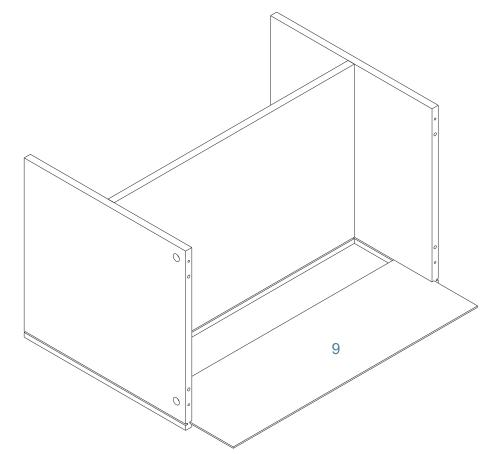
Attach panels[1] to panels[2]. Secure with 6 x bolts(A) as shown. Tighten with allen key (B).
