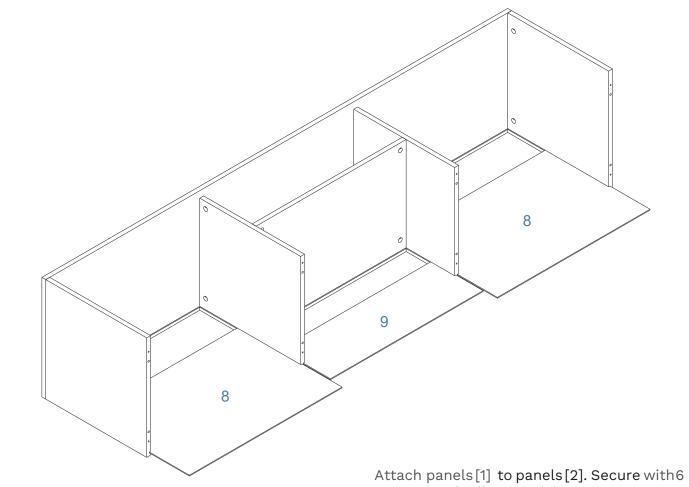
Attach panels[1] to panels[2]. Secure with 6 x bolts(A) as shown. Tighten with allen key (B).
