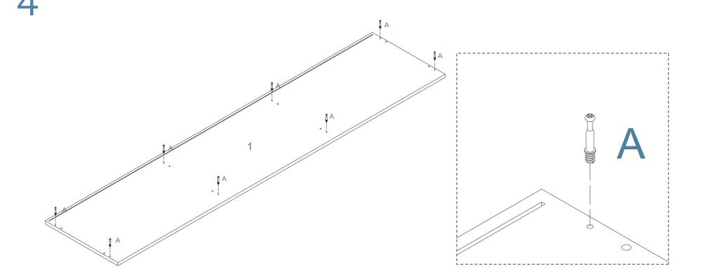
Attach panels[1] to panels[2]. Secure with 6 x bolts(A) as shown. Tighten with allen key (B).
